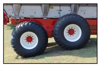
Tandem Axle Walking Beam Suspension:
